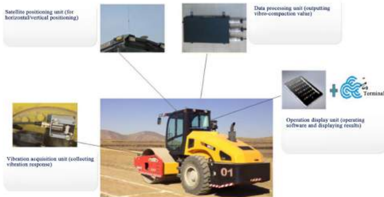
Intelligent subgrade filling
