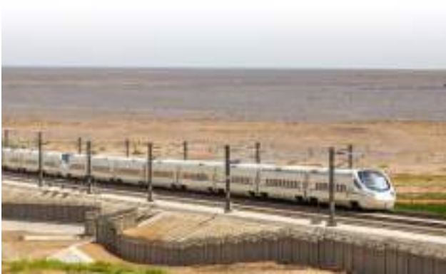
A6 Lanzhou-Urumqi HSR: In December 2014, the Lanzhou-Urumqi HSR, with a total length of 1,776 km and a design speed of 250 km/h, was put into operation. It was the world's longest HSR built in a single project phase and passes through the Gobi desert and strong wind areas.
