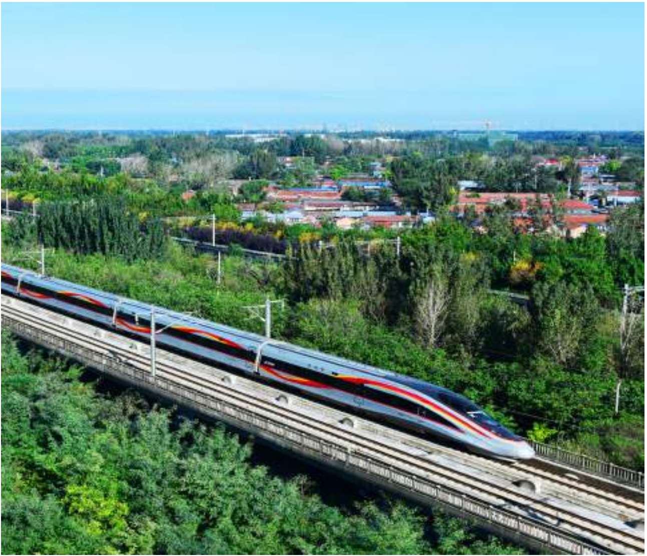
A3 Beijing-Shanghai HSR: In June 2011, the 1,318-km-long Beijing-Shanghai HSR, with a design speed of 350 km/h, was put into operation. It is the busiest HSR line in China.
